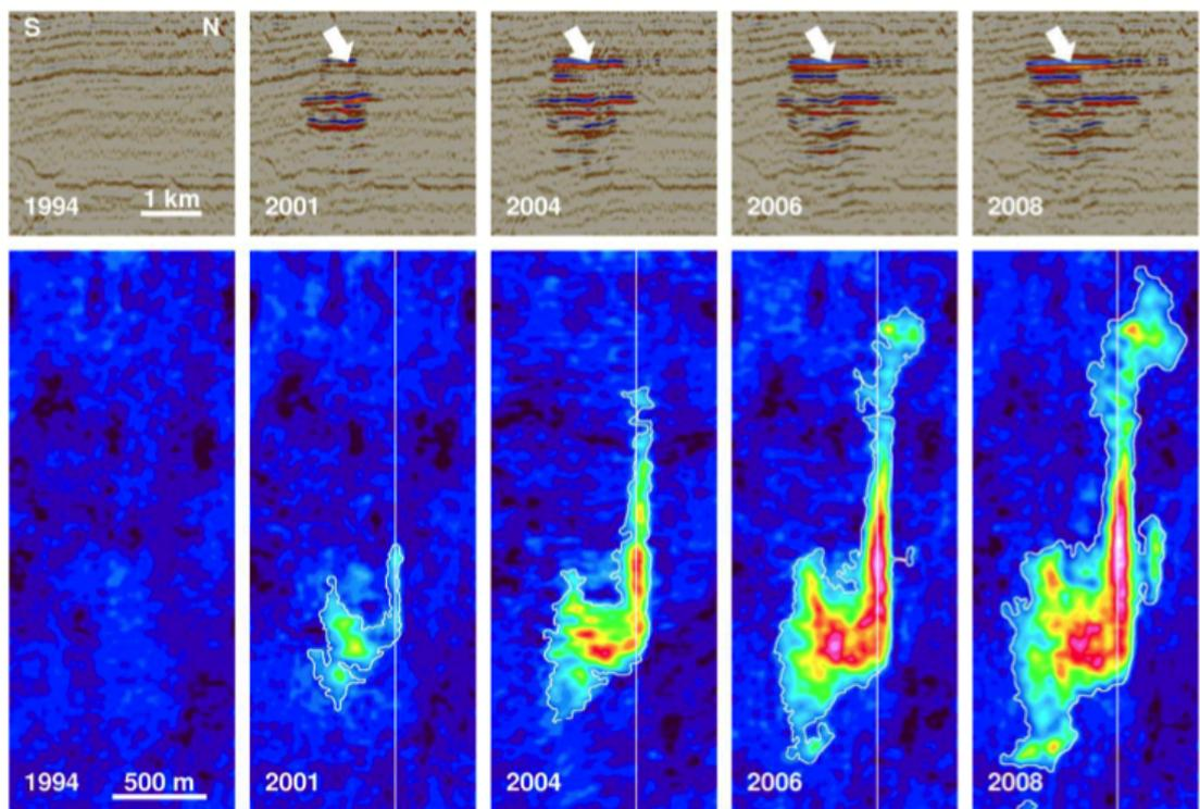
Figure 1: A cross section from successive time-lapse seismic surveys at Sleipner (upper panel) and the total reflection amplitude of the expanding topmost layer in plan view (lower panel).
