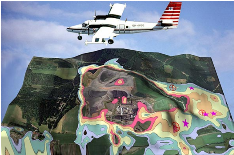
Above: Aerial surveys reveal magnetic and radiometric data of the subsurface.
